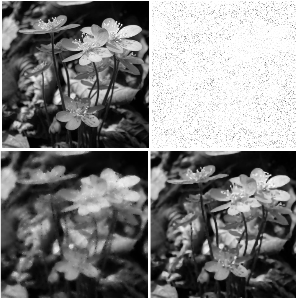
Figure 4.3. Top left: Original image. Top right: 95% random data loss. Bottom left: Inpainted with TV_\epsilon , SSIM: 0.7512. Bottom right: Inpainted with elastica, SSIM: 0.8896.
