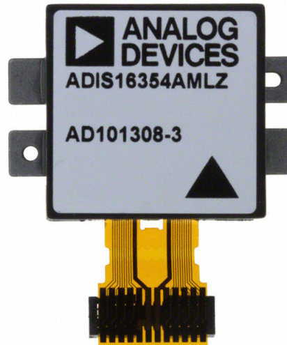
Figure 2.4: Analog Devices ADIS16354AMLZ IMU, (2.3 x 2.3 x 2.3 cm) @ 16 grams.
