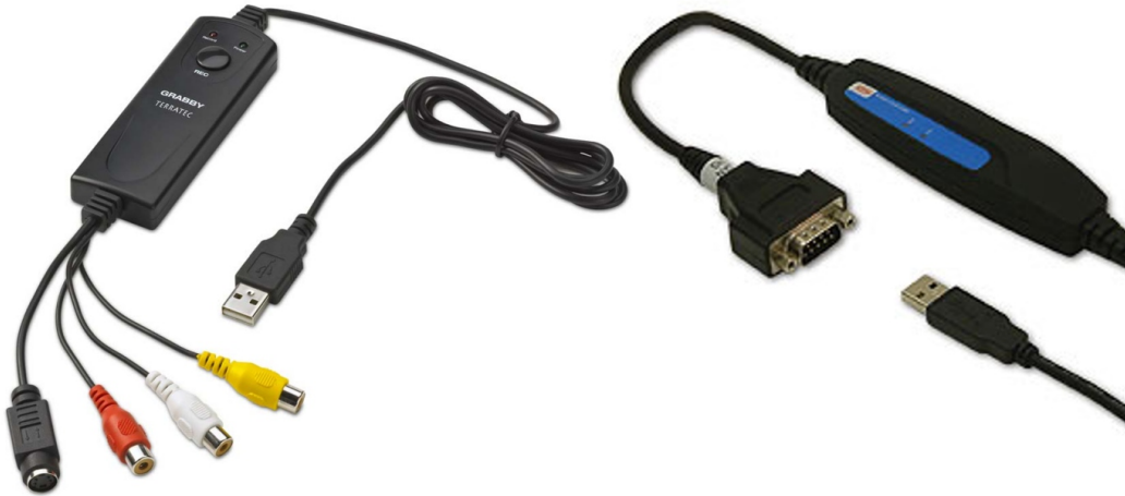
Figure 6.5: TerraTec Grabby on the left and Kvaser Leaf SemiPro HS on the right.
