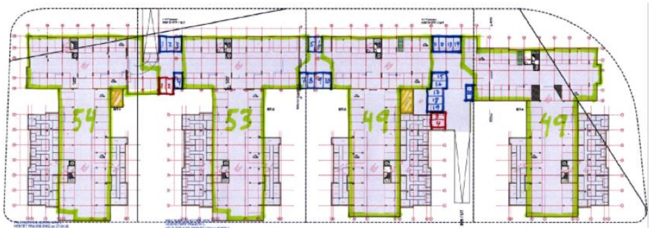
Figure 2: Schematic drawing of four underground garages. The two contrasted in the current analysis are number "54" and "53".
