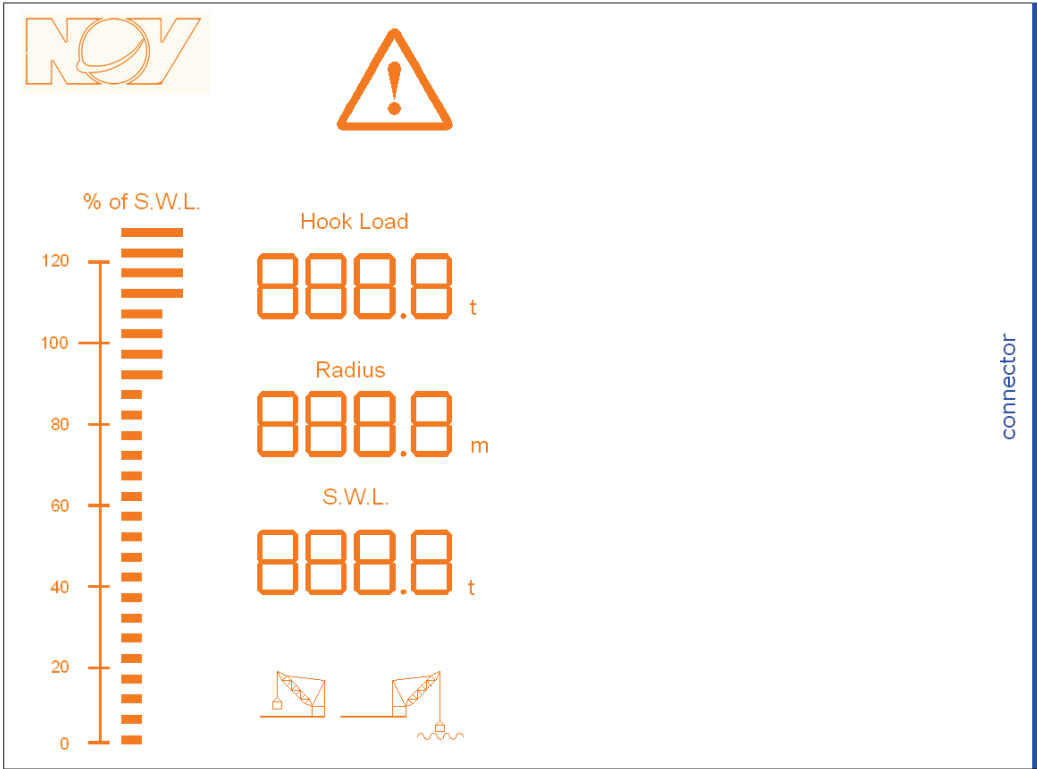
Figure 4-3: Advanced crane operator panel
