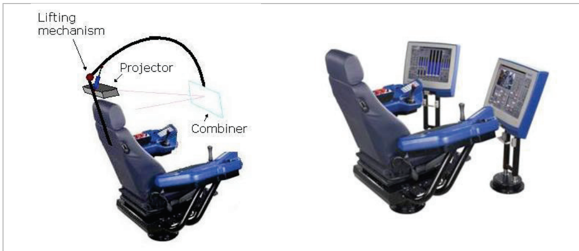
Figure 2-2: Example of a possible way to install a HUD, compared to the existing solution of the same workstation. The HUD can replace one or more LCD screens, or be a useful addition to the HMI. The lifting mechanism is used to raise the combiner and ease entering of the workstation (7).
