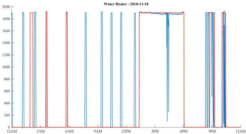
Figure 5.11: Parson: Water Heater consumption and detection on day 14.
