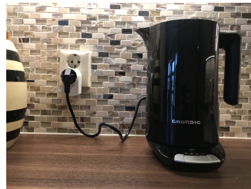
(c) Raspberry Pi B+ in case with Plugwise Stick (d) Plugwise Circle connected to an electric kettle.
