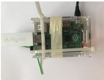
(c) Raspberry Pi B+ in case with Plugwise Stick (d) Plugwise Circle connected to an electric kettle.
