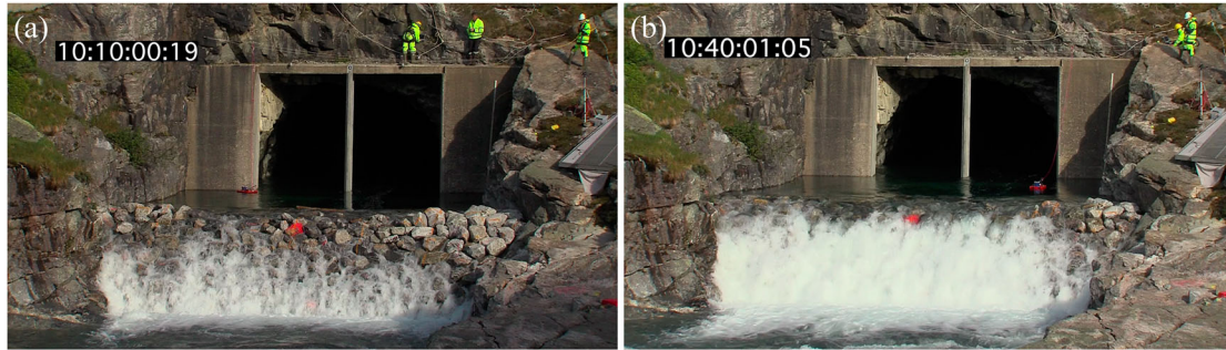
Figure 5. Picture frames of the test F15D1 with dumped riprap: (a) partly overtopped test dam with most of discharge as through flow q = 0.2 \text{ m}^2\text{s}^{-1} ( F_s = 0.3 ); (b) cascading flow at q = 0.4 \text{ m}^2\text{s}^{-1} ( F_s = 0.6 ). (Video: S. R. Skilnand).
