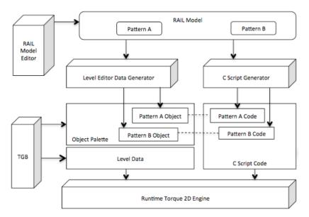
Fig. 3. The Tool Chain Architecture for RAIL Modeling with Torque 2D
