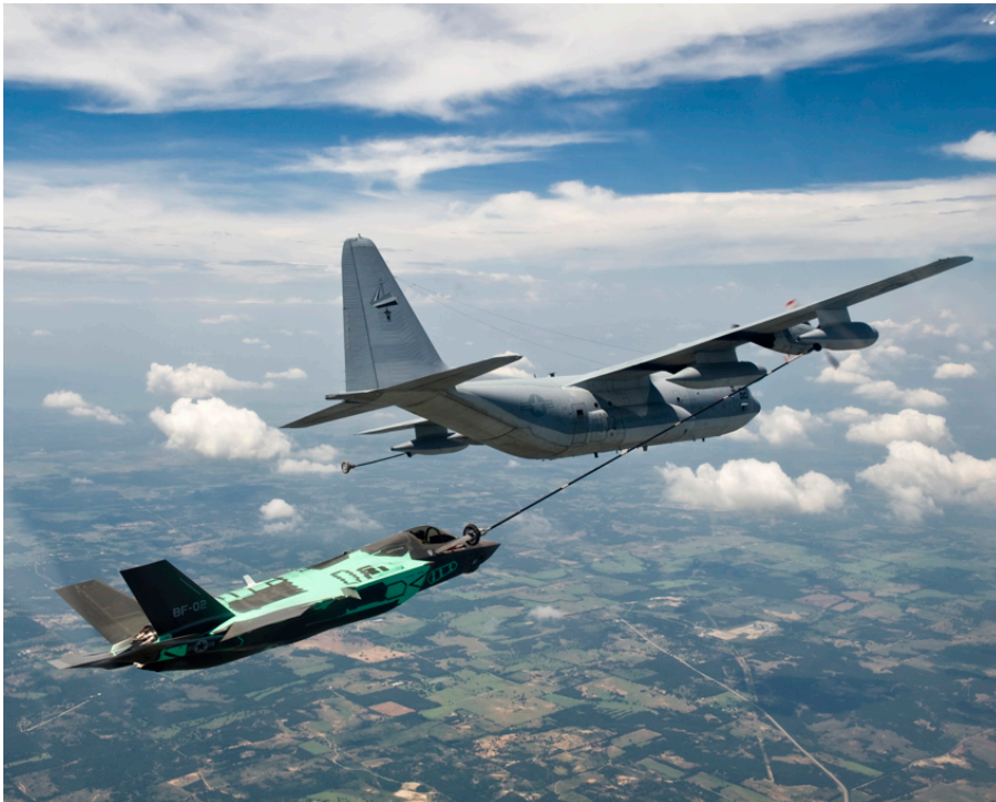
Figure 1.6: The first aerial refuelling including F-35 Lightning II stealth fighter. Courtesy of Lockheed Martin, http://www.lockheedmartin.com .
