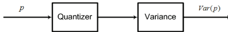
Figure 3.5 – Shows how variance is computed in the Simulink model. The variance block needs a quantized input in order to function.
