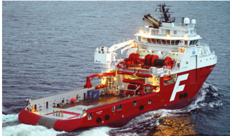
Figure 2.1. Far Sapphire Anchor Handling Tug and Supply Vessel. Photo courtesy to Farstad .
