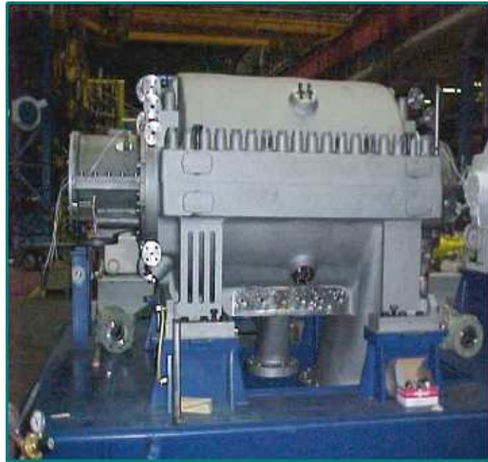
Figure 1.2: Centrifugal compressor with horizontally split outer casing. (Siemens, 2008).
