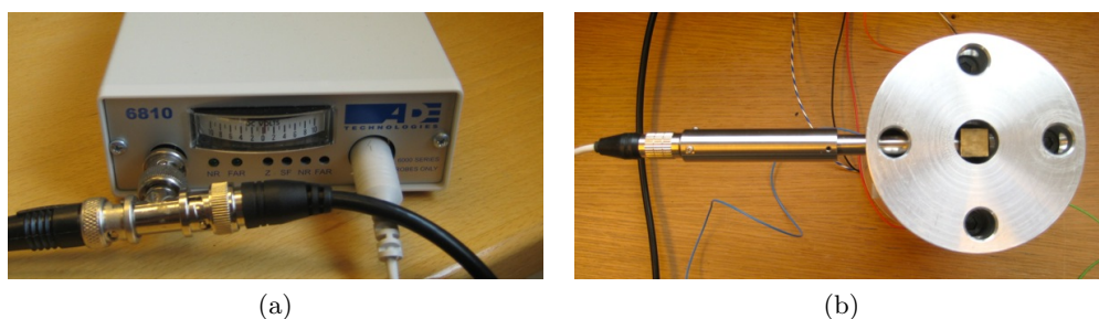
Figure 3.7: Photos of the capacitive sensor a) gauge, b) probe and target.
