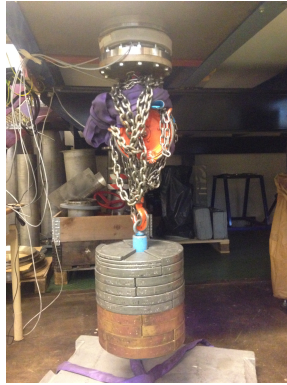
Figure 3.5: Experiment setup for loads below 200\text{kg} .
