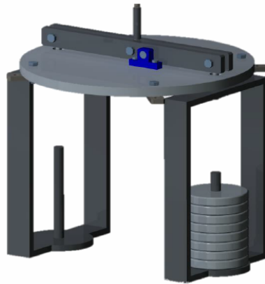
Figure 3.8: Axial force calibration system. [8]
