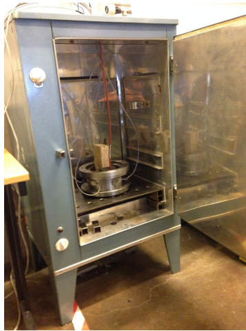
Figure B.1: The ALMD placed in the heating cabinet.
