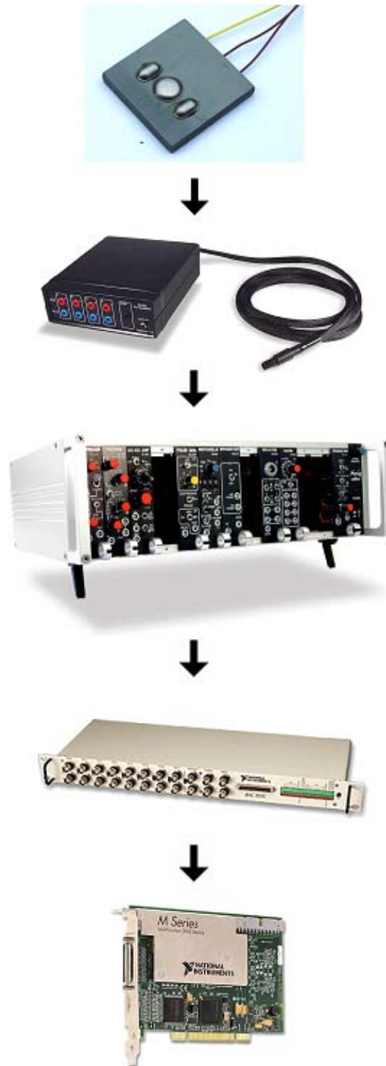
Figure 5: Signal processing equipment. Myoelectrode - NL844 - NL900D - BNC-2090 - PCI6251 (from top to bottom)
