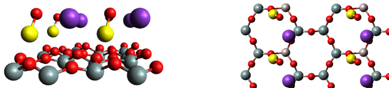
Figure 4.7: The structure of ZnO-mica, with zinc coloured yellow.
