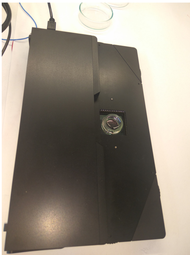
Figure 3.6: The headstage with an MEA inserted.
