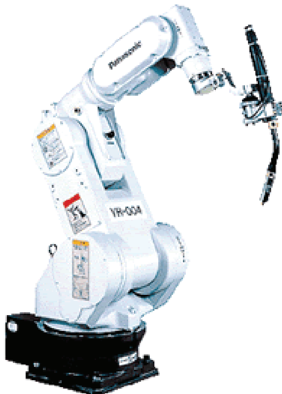
Figure 2.1: A Panasonic robotic welder with 6 Degrees of freedom(DOF).
