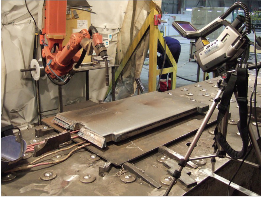
Figure 8.1: The rig set-up, with the camera in front, the steel plate on the work bench and the manipulator behind.
