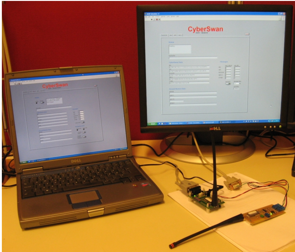
Figure 6.1: Hardware setup for HIL test.
