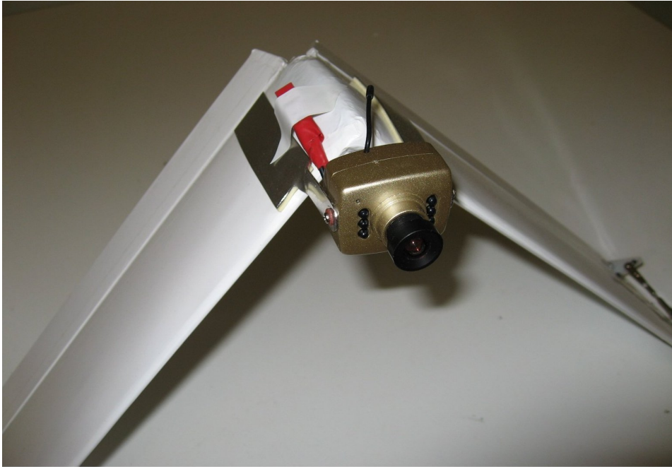
Figure 5.5: Minikameran mounted on the CS's back wing.
