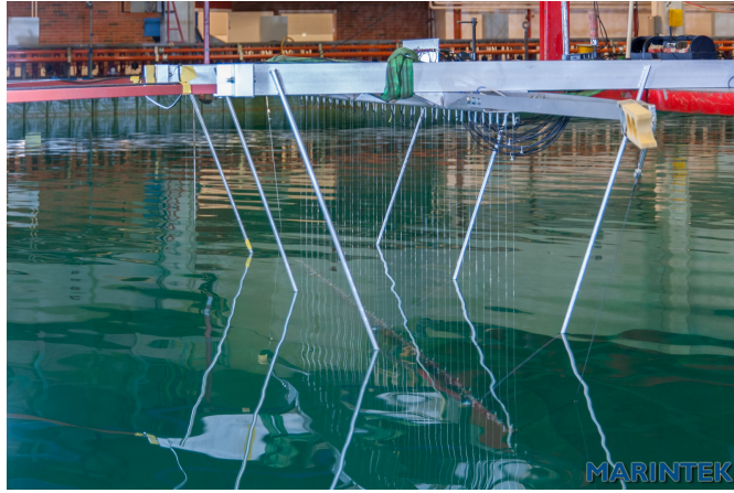
Figure 4: Wave harp as installed during wave calibration.
