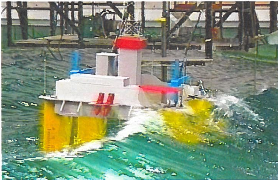
Figure 1.1: Model test of semi-submersible in extreme waves.
