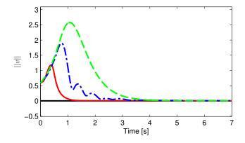
Fig. 5. System states' norm ||v|| in the state-feedback (solid red) and output-feedback cases of Theorems 7 (dashed-dotted blue) and 8 (dashed green).
