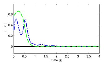
Fig. 7. Observer estimation error norm  $||v - \hat{v}||$  when using the controllers of Theorems 7 (dashed-dotted blue) and 8 (dashed green) with faster convergence times.
