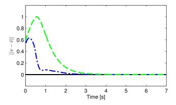
Fig. 6. Observer estimation error norm  $||v - \hat{v}||$  when using the controllers of Theorems 7 (dashed-dotted blue) and 8 (dashed green).
