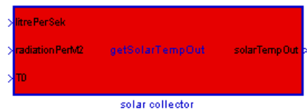
Figure 3.8: Solar collector functionality in embedded Matlab block
