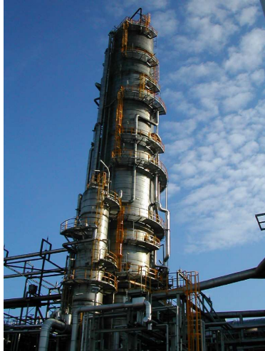
(a) Picture of a crude oil distillation column (Wilhelmshavener Raffinerie Gesellschaft, 2004).
