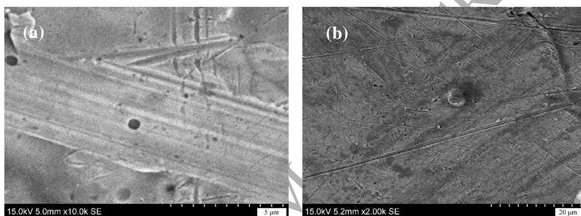
**Fig. 9.** SEM surface morphology of the gold current collector (a) before and (b) after the thermocell measurements.
