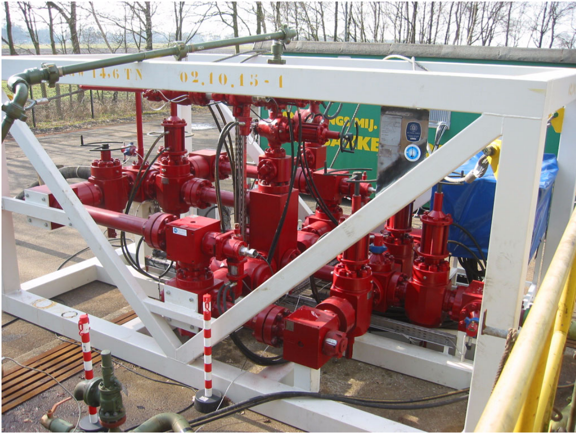
Fig. 2a. Custom built choke manifold installed on test site with control cabin in background.
