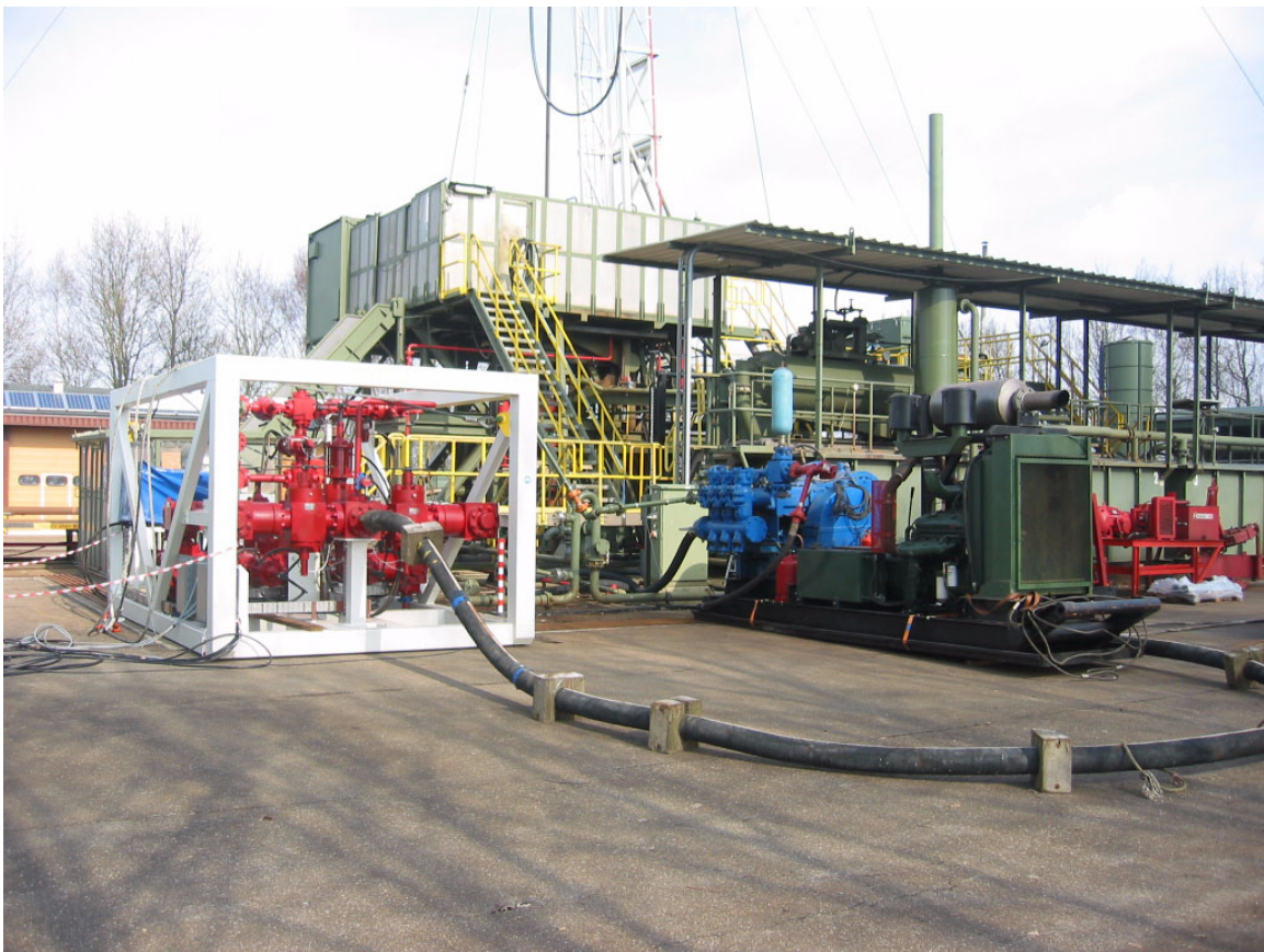
Fig. 2b: Choke manifold and back-pressure pump installed on SimWell test facility.
