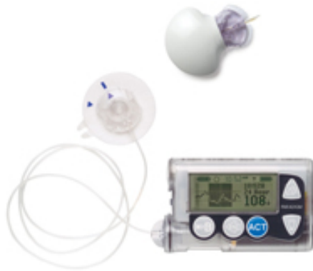
Figure 5: Combined continuous glucose monitor and insulin pump from Medtronic. The sensor (located on the upper white device in the picture) is placed in the subcutaneous tissue, and measurement signals are transmitted wirelessly to the monitor.
