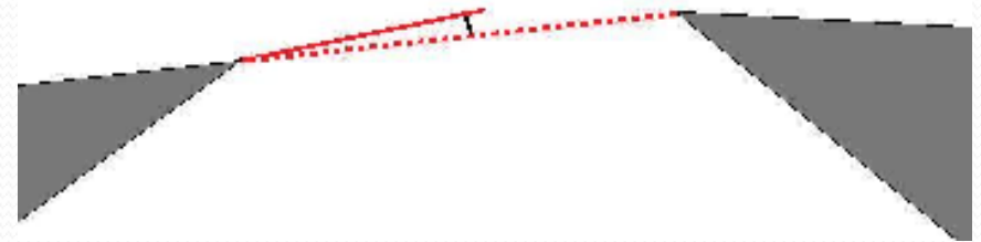
With similar heaves, an increase in ramp length directly reduces pitch as seen in old pitch (solid line) to new pitch angle (dashed line)
