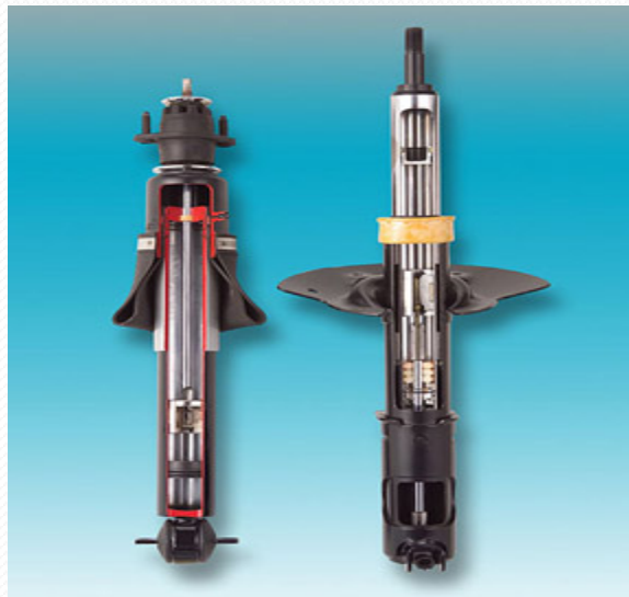
Shock absorber (right) and Suspension strut (left) Delphi Corporation
