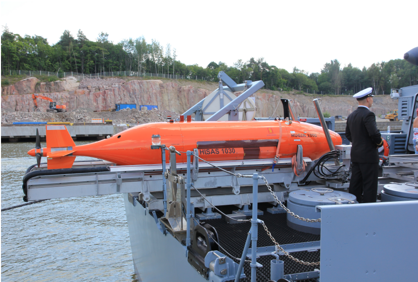
Figure 1.2: Hugin 1000 AUV on board a ship. Illustration from Wikipedia under public domain.
