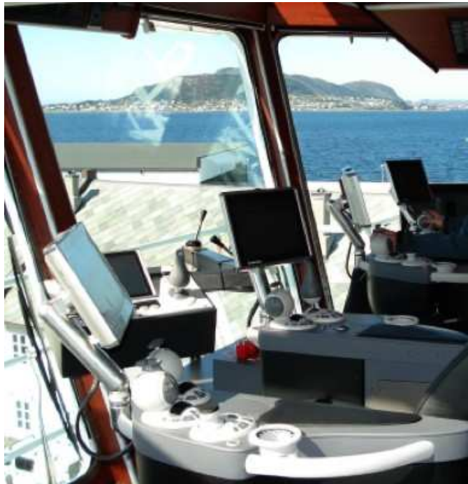
Figure 1.2: Rolls-Royce Marine DP operator station on the supply vessel Volstad Viking. Courtesy of Rolls-Royce Marine AS.
