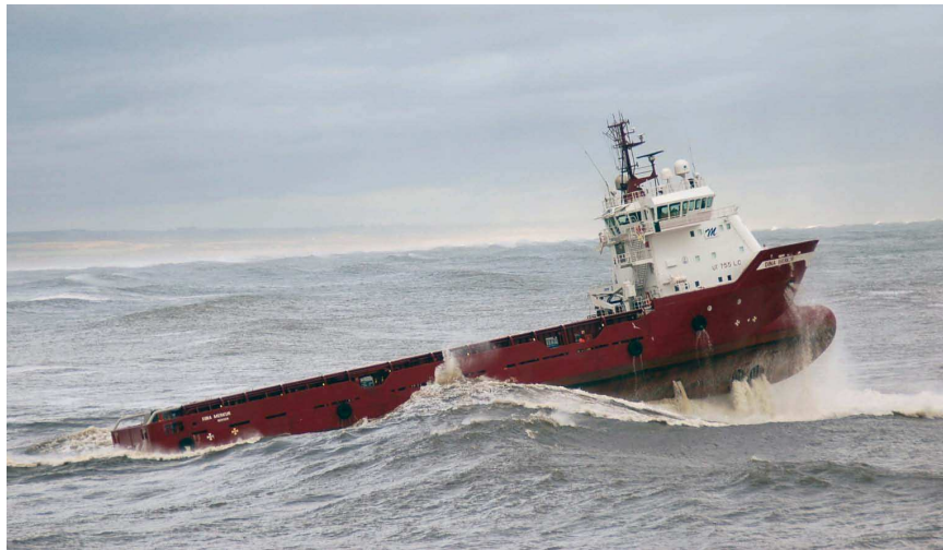
Figure 5.10: A supply vessel in sea state condition upper 5 outside Aberdeen, Scotland. Courtesy of Rolls-Royce Marine AS.
