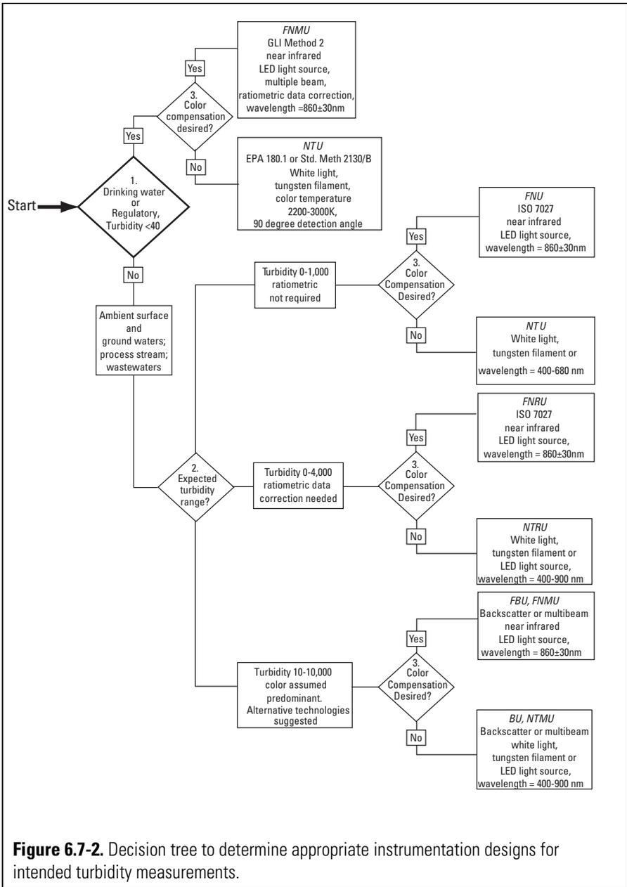
**Figure 6.7-2.** Decision tree to determine appropriate instrumentation designs for intended turbidity measurements.
