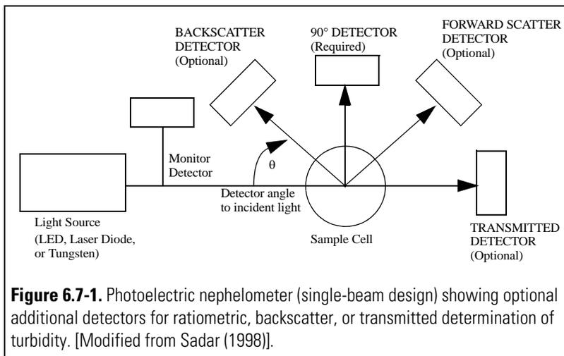
**Figure 6.7-1.** Photoelectric nephelometer (single-beam design) showing optional additional detectors for ratiometric, backscatter, or transmitted determination of turbidity. [Modified from Sadar (1998)].
