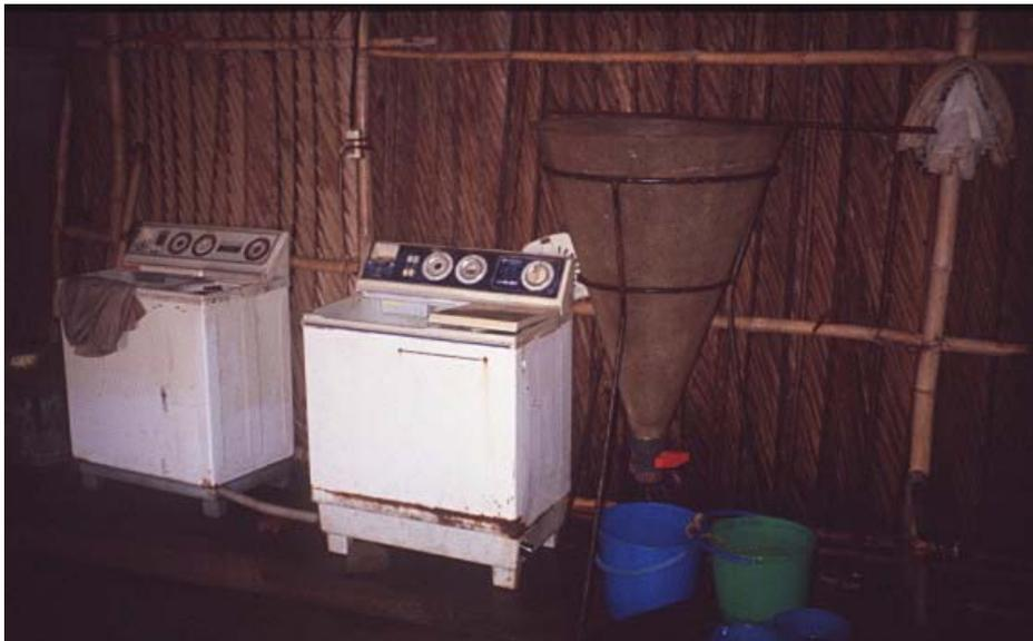
**Figure 4.5.27. A vertical spin dryer (for removal of excess water) and a transparent conical shaped tank with a bottom valve (for density separation).**
