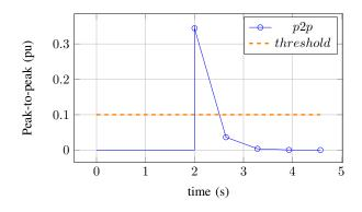
Fig. 2. Outer bounds detected oscillation magnitude.
