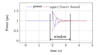
Fig. 1. Example of a ring-down signal.
