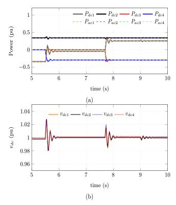
Fig. 5. Normal HVDC grid behavior, (a) power signals and (b) voltage signals at each node.
