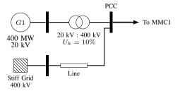
Fig. 3. Topology of ac grid at node 1.
