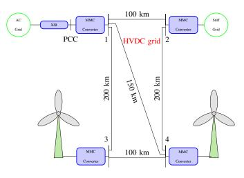
Fig. 4. Multiterminal HVDC grid.
