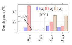
Fig. 10. Damping ratio of the oscillations detected with the abnormal behavior for the DC power.
