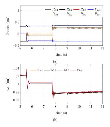
Fig. 6. Abnormal HVDC grid behavior, (a) power signals and (b) voltage signals at each node.
