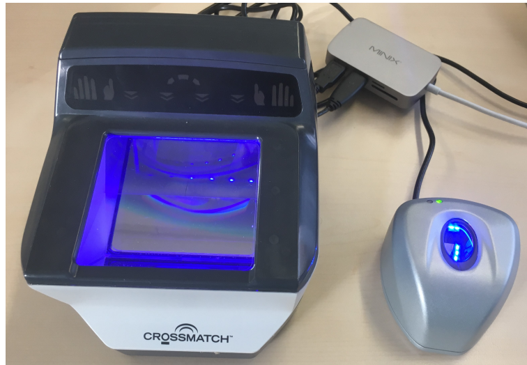
Figure 32: Crossmatch Guardian 200-Rev 1 sensor on the left side and Lumidigm v203 on the right side
