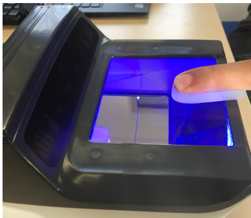
(a) Dragon-skin fake finger PA performed on Crossmatch sensor
