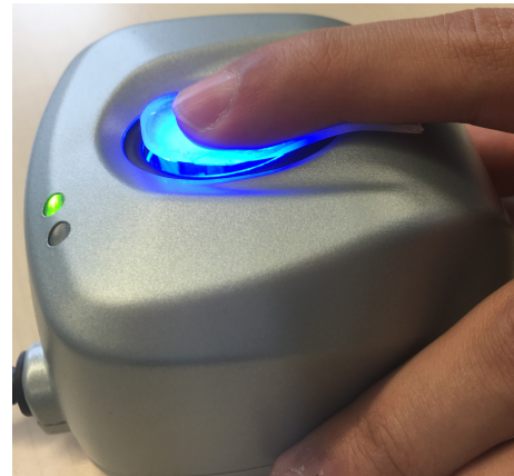
(b) Silicone overlay PA performed on Lumidigm sensor
