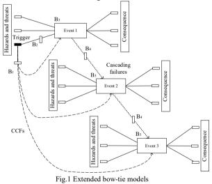
Traditional risk analysis defines often the first departure from normal operation as a *trigger event*. For example, [41] defines a triggering event as "an event or condition that is required for a hazard to give rise to an accident". Translated into the context of CCFs and cascading failures, we may consider the triggering events as root causes.
