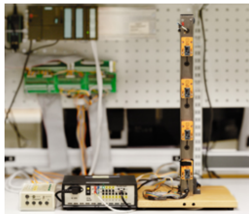
Fig. 3. The elevator model setup used in the course project. Courtesy of the Dept. of Engineering Cybernetics, Norwegian University of Science and Technology (NTNU), Trondheim, Norway.
