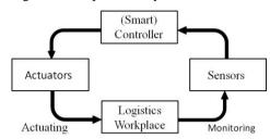
Fig. 1. A Smart Closed-loop System for Workplace Safety
