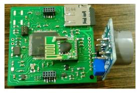
Fig. 2. WSN sensor units for CO2, with alternative communication module
