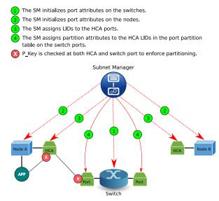
Figure 1: Partition validation process in IB networks.
