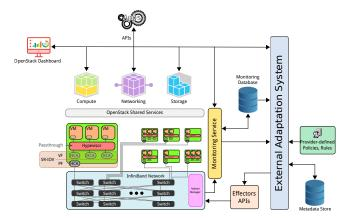
Figure 2: Architecture overview of a self-adaptive HPC cloud based on OpenStack and InfiniBand interconnect.
