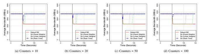
Figure 7: Average flow bandwidth for different weight calculation methods and historical counters.
