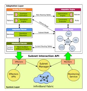
Figure 3: A self-adaptation framework for IB subnets.
