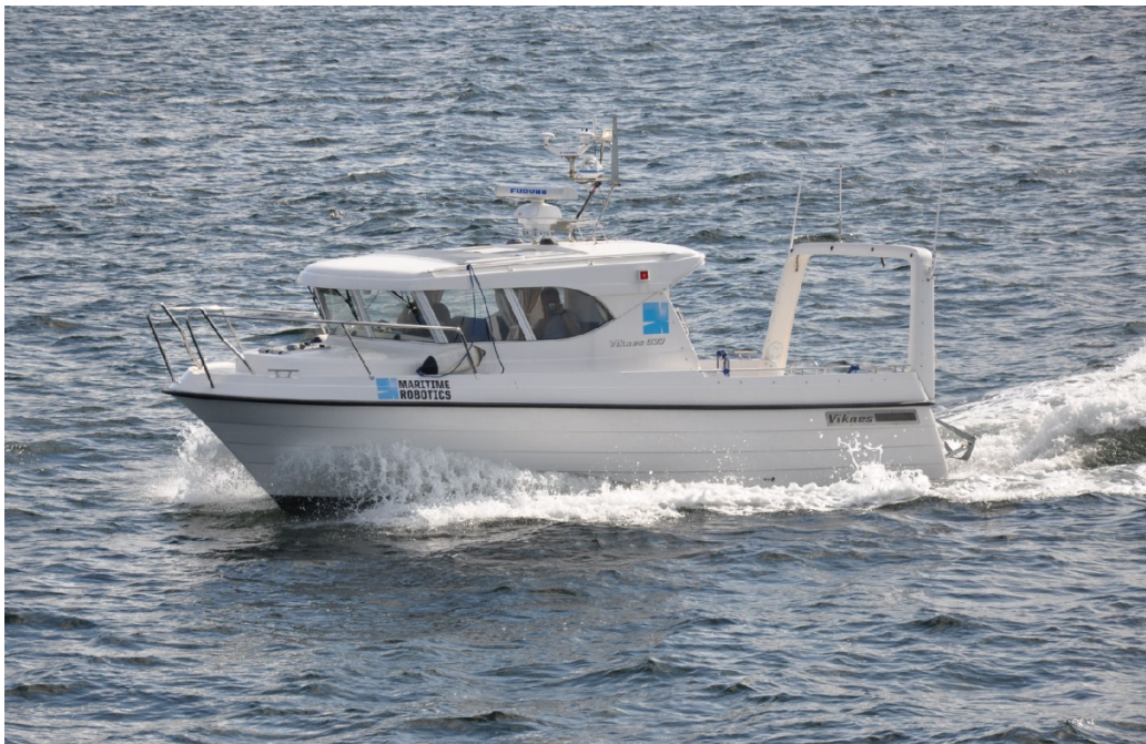
Figure 36: The Viknes USV represents a flexible test platform from which to conduct full-scale motion control experiments throughout the year. Courtesy of Maritime Robotics.
