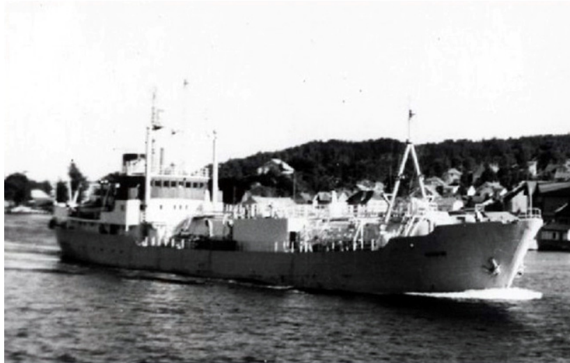
Figure 4: Norsk Hydro's ammonia tanker M/S Haugvik was retrofitted with experimental automation technology to enable unmanned engine rooms. Courtesy of DNV.
