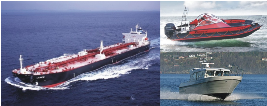
Figure 23: As seen to the left, a large oil tanker is an example of a displacement vessel, while a semi-displacement leisure boat is seen to the bottom right and a RIB-type planing vessel to the top right.
