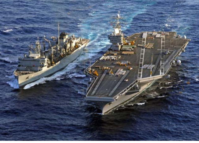
Fig. 1. Two naval ships performing underway replenishment; the guide ship to the left and the approach ship to the right. Courtesy of the US Navy.
