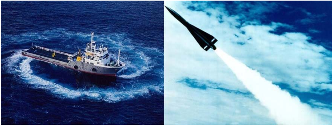
Figure 14: A ship rotating around its vertical axis and a surface-to-air missile just after launch. Ships maneuvering at low speed are often fully actuated, but missiles are inherently underactuated.
