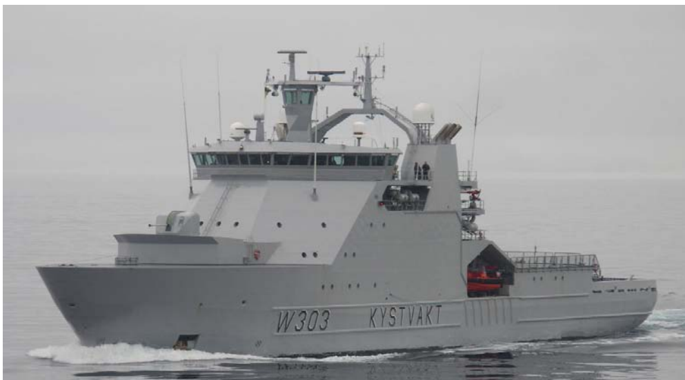
Figure 11: KV Svalbard is a Norwegian coast guard vessel which operates mostly in Arctic waters. Similar to the Orions, its capacity can be expanded through the use of unmanned surface vehicles (USVs) and unmanned underwater vehicles (UUVs). Courtesy of the Royal Norwegian Navy.
