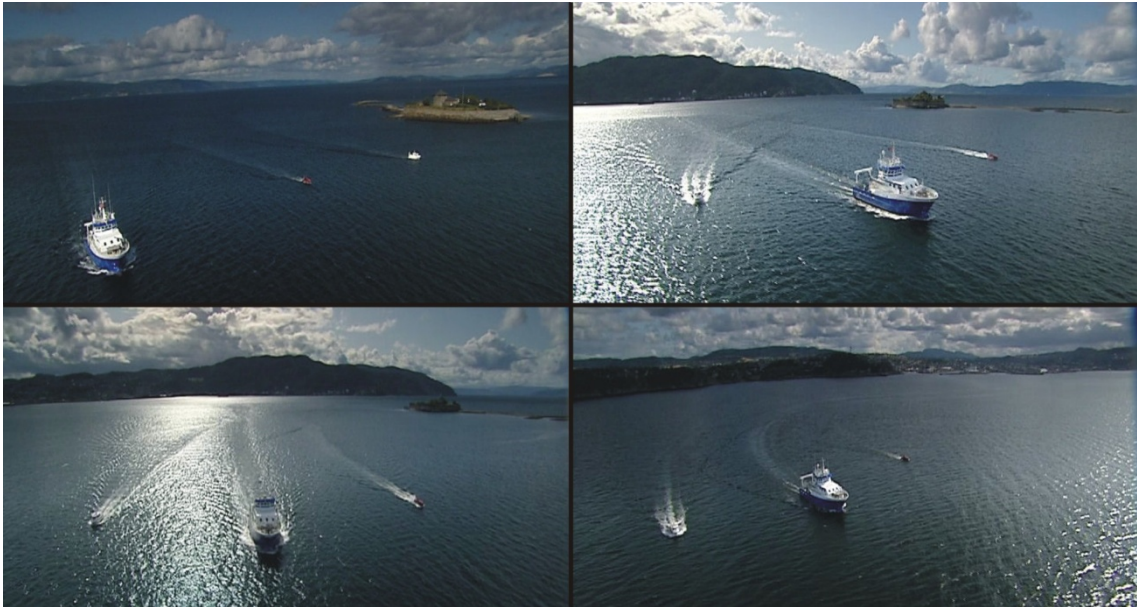
Figure 46: The top left photo shows the two USVs both travelling in formation on Gunnerus' port side; the top right photo shows the Viknes USV changing its formation position to starboard of Gunnerus; the bottom left photo shows the new formation configuration where the two USVs travel on different sides of the leader vessel; while the bottom right photo shows that the formation geometry is kept even when Gunnerus executes a circular maneuver. Photos courtesy of NRK.
