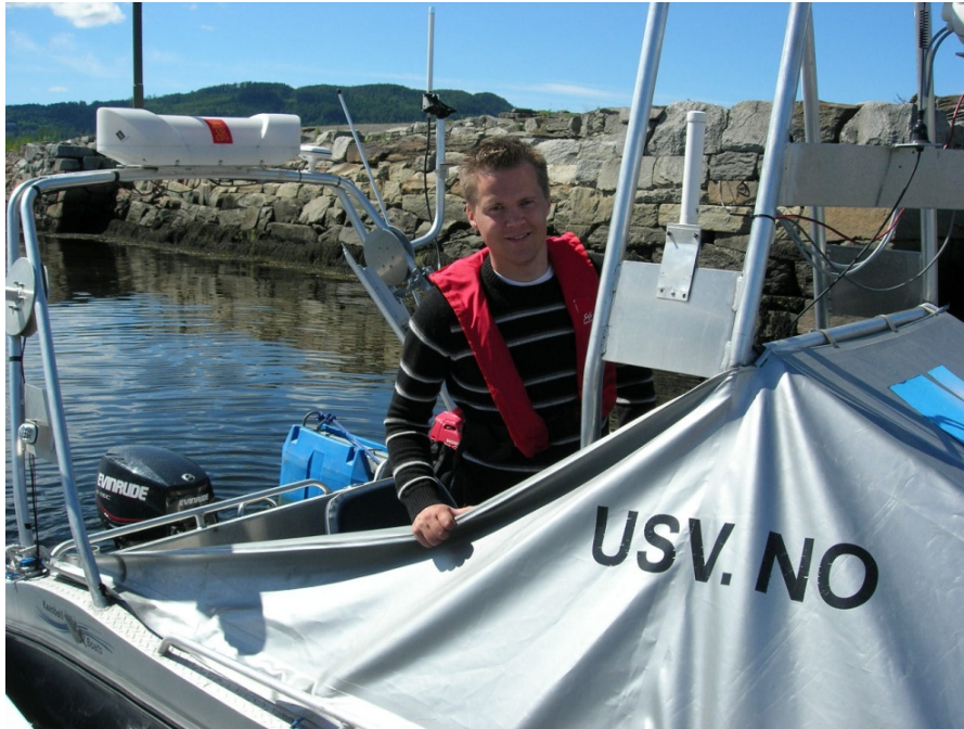
Figure 35: Initial sea trials with target tracking were carried out in June 2008 with a retrofitted Kaasbøll 19-foot planing monohull equipped with an Evinrude 50 E-Tec outboard engine.
