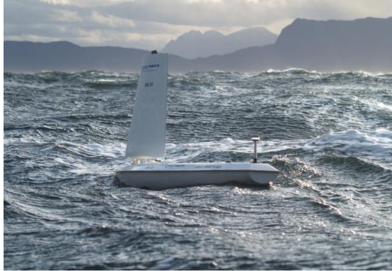
Figure 34: A two-meter long sailing buoy intended for collection of meteorological and oceanographic data in areas where traditional buoy technology falls short. Courtesy of CMR.
