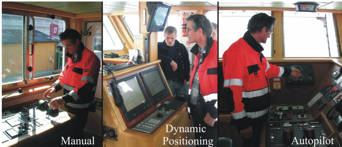
Figure 50: Today, the captain of a well-equipped vessel usually has at least 3 different modes of operation from which to choose. With an integrated motion control system, the dynamic positioning and autopilot functionalities could be merged into a single functionality covering all vessel speeds.
