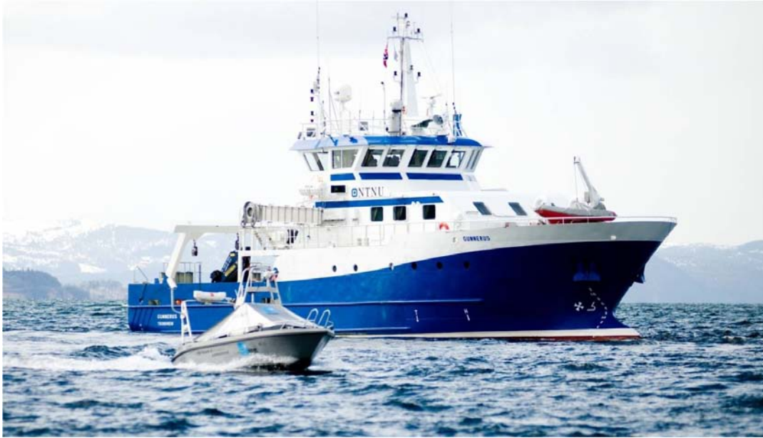
Figure 42: NTNU's research vessel Gunnerus is a 30 m long displacement vessel capable of reaching a maximum speed of 13 knots. The phased-out Kaasbøll USV is seen in the foreground. Courtesy of Maritime Robotics.
