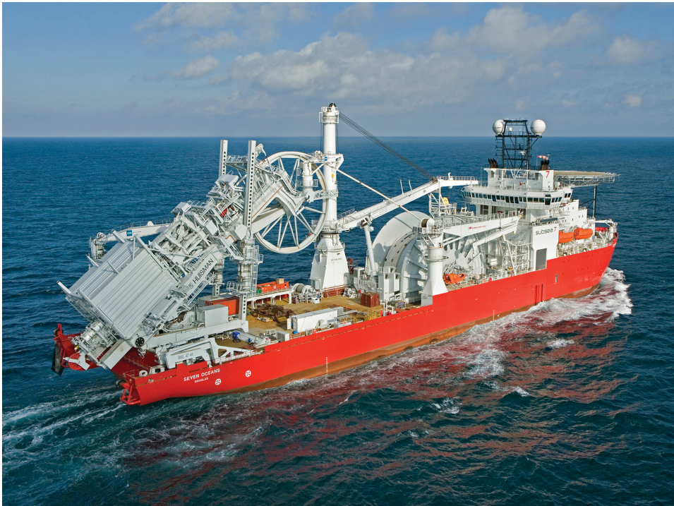
Figure 2.6: Seven Oceans owned by Subsea 7 is a pipelaying– and offshore construction vessel, delivered in 2007, capable of installing 16 inch pipelines in depths reaching 3000 meters. Huisman–Itrec ( www.huismanequipment.com ) designed and built the complex pipelay installation on the ship. Behind the superstructure a reel with a weight of 950 tonnes has been integrated in the ship. This reel can store up to 3500 tonnes of rigid steel pipe. Courtesy of Subsea 7.
