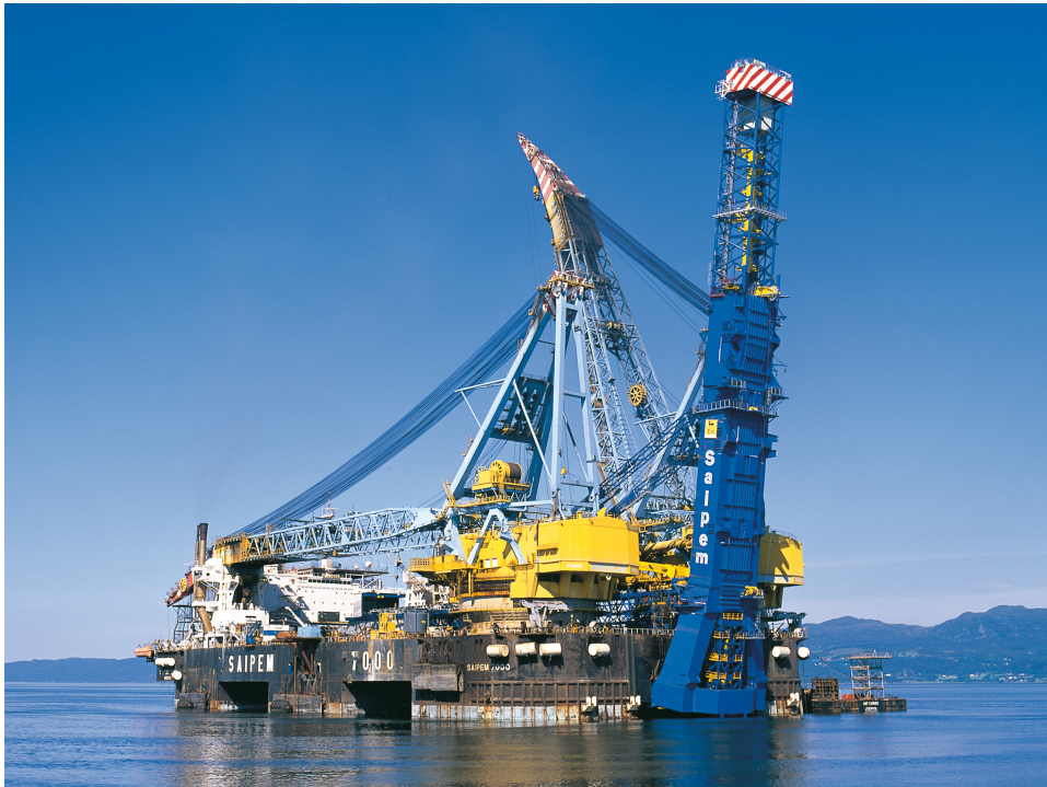
Figure 2.5: Saipem 7000 owned by Saipem is a semisubmersible crane vessel that has been in operation since 1998. During the winter of 1999–2000 the vessel underwent a refit to enhance its positioning and power systems and add a J-lay system. The J-lay tower can lay pipe from 4” to 32” diameter with a tension of up to 525 tonnes (5.15 MN) using the tensioners and up to 2,000 tonnes (20 MN) when using friction clamps. Courtesy of Saipem SpA.
