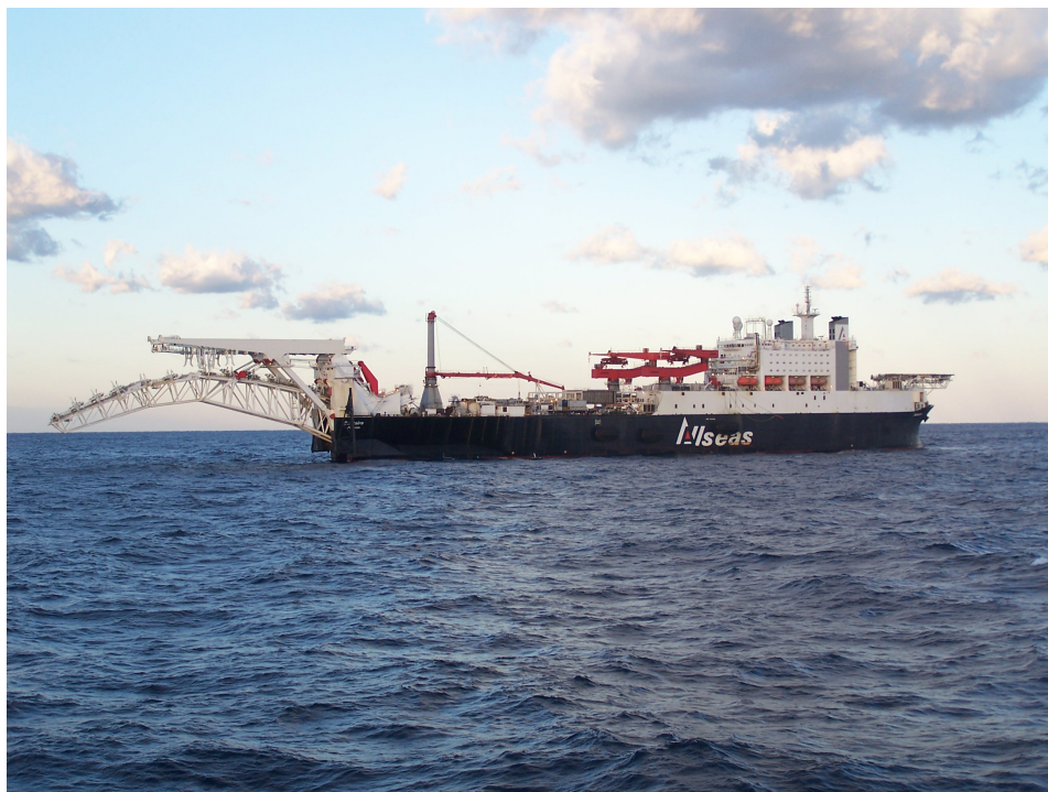
Figure 2.4: Solitaire , the largest S-lay vessel in the world, 300 m (984 ft) excluding stinger. Her S-lay capacity was increased in 2005 to a holding force of 1050 t, enabling her to lay the heaviest pipelines. Courtesy of The Allseas Group.
