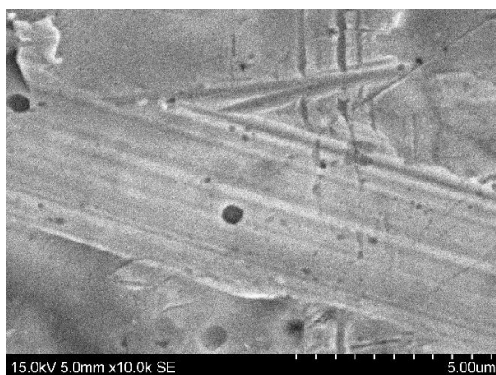
Figure 3.2.8 SEM surface morphology of the gold electrodes before thermocell measurements.
