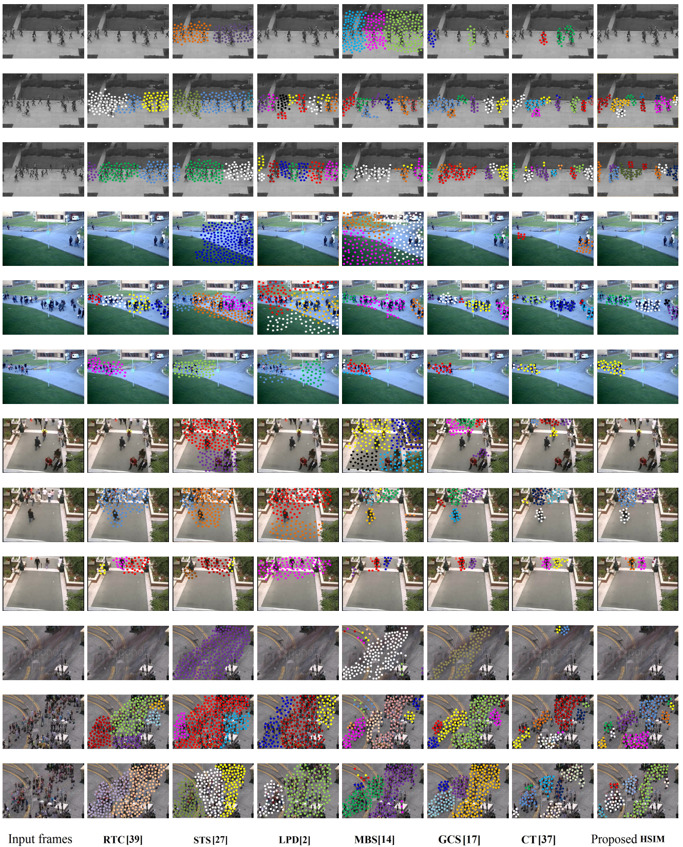
Fig. 8 Qualitative comparison. The proposed HSIM method is compared with two baseline: RTC [39] and STS [27], and four state-of-the-art: LPD [2], MBS [14], GCS [17], and CT [37] motion segmentation methods. The top three rows represent frames from UCSD dataset, the next three rows represent frames from PETS2009 dataset, the second last three rows represent frames from USC dataset, and the bottom three rows represent frames from CUHK dataset. The last column shows that our proposed HSIM method performs accurate segmentation.
