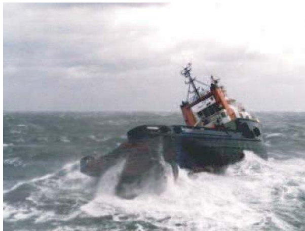
Figure 4.3: A ship in extreme sea conditions. An anti-spin protection is needed in order to prevent the propeller from spinning when experiencing ventilation and in-and-out-of-water effects.
