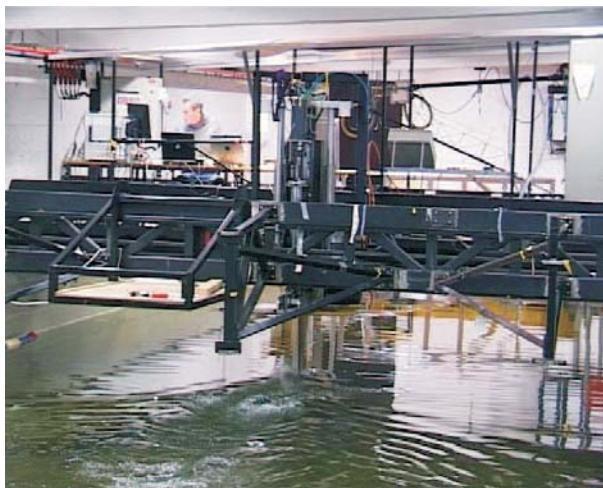
Figure 5.3: A test setup in MCLab at NTNU. The LTC for transit operation in extreme sea conditions with integrator reset was tested in a basin. The nonzero advance speed was effectuated by moving the thruster horizontally using a towing carriage. Also the thruster vertical position was moved in order to trigger ventilation and in-and-out-of-water effects.
