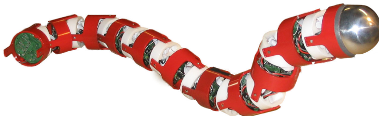
Figure 7.1: The NTNU/SINTEF snake robot ‘Aiko’.
