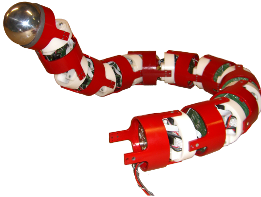
Figure 1.3: The snake robot ‘Aiko’ developed at the NTNU/SINTEF Advanced Robotics Laboratory. Aiko is used as a basis for the mathematical models.
