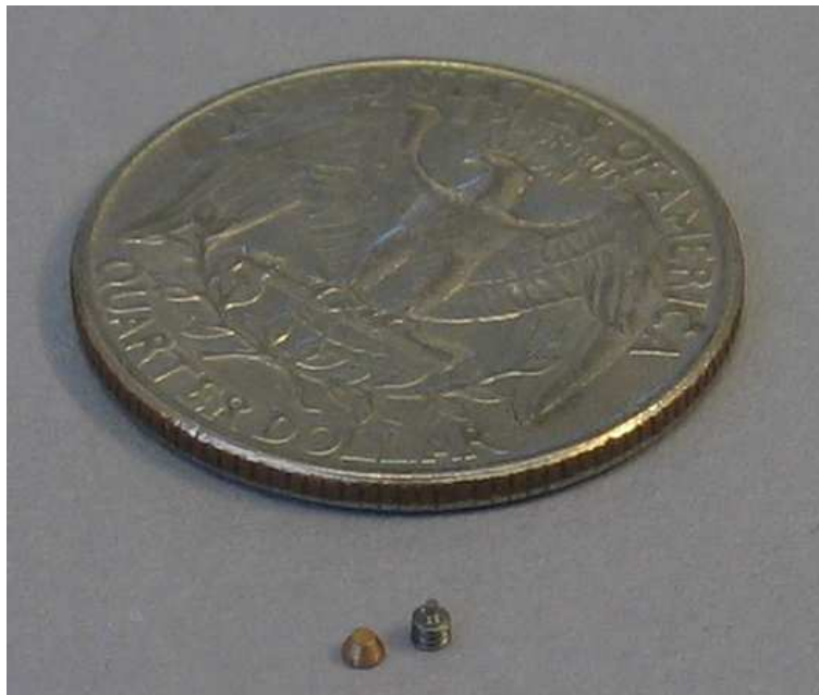
Figure 6.4: The adaptive pin shape, where the right part shows the screw with a ball joint, and the left part is the actual tactel top.
