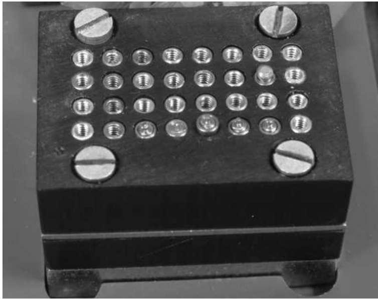
Figure 5.5: Figure showing the display housing. Five of the tactels in the front row have a pointed pin shape, while one of the tactels in the third row has a round pin shape.
