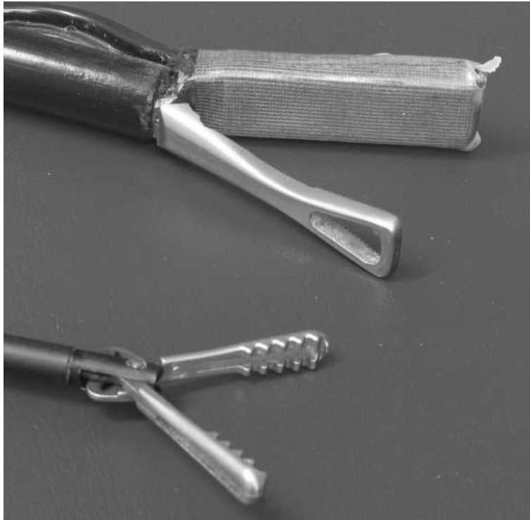
Figure 7.14: Figure showing the end effectors of LIT at the top and a conventional laparoscopic grasper (LI) at the bottom.
