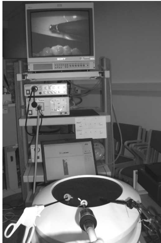
Figure 4.4: Experiment setup when laparoscopic instrument with sensor was used (the laptop behind the surgical simulation trainer presents the pressure distribution visually).
