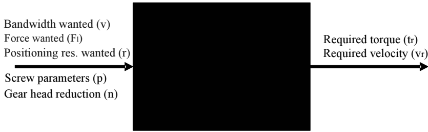
Figure 5.16: "Black box" parameters for finding required torque and velocity.
