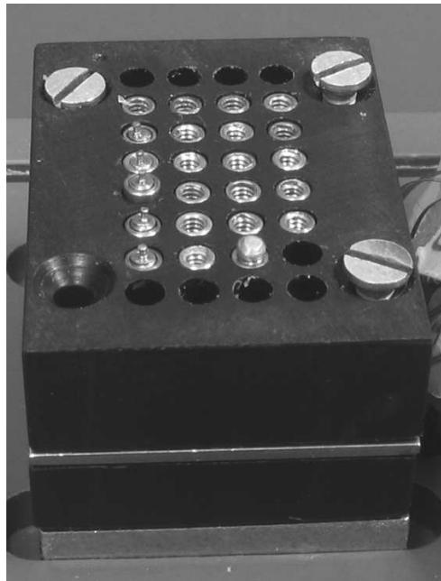
Figure 6.1: Tactile display with 23 tactels mounted. The left column shows pointed pins. In the front row the adaptive shape is shown. The rest are blunt pins.
