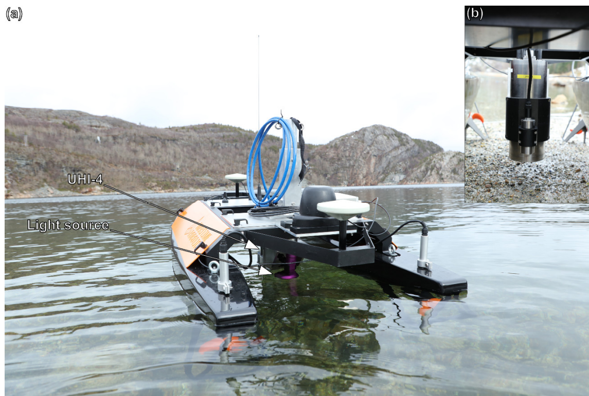
Figure 2. The OTTER USV (unmanned surface vehicle) after deployment in Hopavågen (63°35′N 9°32′E), Agdenes, Norway (a). The positions of UHI-4 (4th generation underwater hyperspectral imager) and the light source are shown with arrows. Panel (b) shows a close-up photograph of UHI-4.
