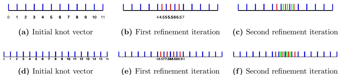
Figure 4.5: 1D Central Refinement: The first three steps of the refinement process in the cases p = 2 (above) and p = 3 (below). When two functions are equally close to the centre, the rightmost one is selected for refinement.
