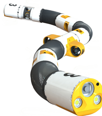
Fig. 1. The Eelume USM, an example of an underwater snake robot. It is approximately 3.3 m long and weighs 80 kg.
