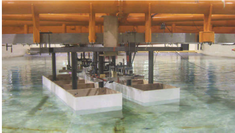
FIGURE 13. (Colour online) Barge models in the tank.
