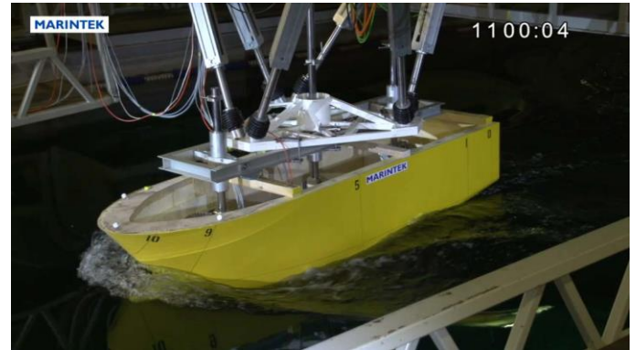
FIGURE 1: PLANAR MOTION MECHANISM TESTS IN TOWING TANK [ Courtesy of SINTEF Ocean [27]]
