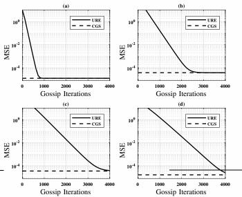
Fig. 4. Comparison of MSE of estimate of the PMU observable states obtained by WAMS for (a)4, (b)7, (c)11, and (d)14 areas when using CGS and URE gossip schemes.
