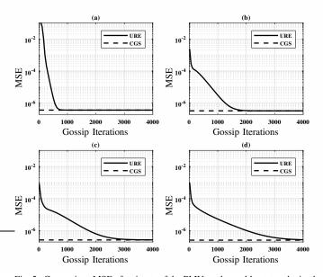
Fig. 5. Comparison MSE of estimate of the PMU unobservable states obtained by reduced order estimator for (a)4, (b)7, (c)11, and (d)14 areas when using CGS and URE gossip schemes.
