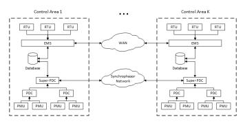
Fig. 1. Monitoring architecture of the smart grid.
