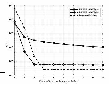
Fig. 2. Performance of the proposed method when compared with the DARSE scheme of [23] with 10 and 50 gossip iterations between Gauss-Newton descent steps.
