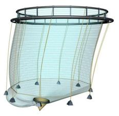
Figure 1: Floating fish farm with circular plastic collar consisting of two tori that are nearly semi-submerged in calm water, railing, jump net, netting, dead fish removal system, frame of ropes and bottom weights. (Sintef Fisheries and Aquaculture).
